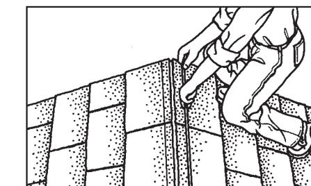
Step 1 – On existing roofs, remove cap shingles. Mark slot width at both ends of ridge. Use slot guides imprinted on vent and refer to drawings on the other side. Snap chalk line on both sides of ridge.
