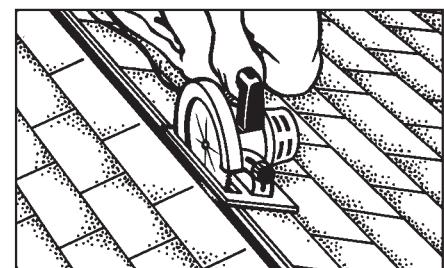
Step 2 – Cut slot (plumb cut, if possible). Note: Adjust depth of blade to avoid cutting rafters or trusses. Refer to drawings for slot dimensions. Remove debris from slot.
