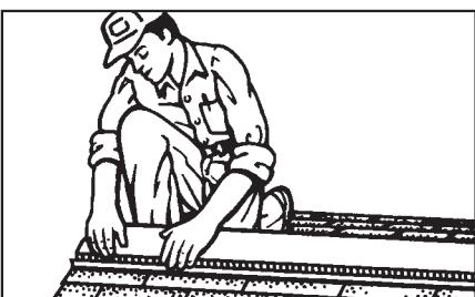
Step 5 – Nail cap shingles in place using roofing nails long enough to penetrate the underside of the roof.
