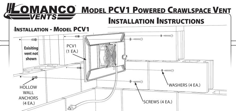
The PCV1 requires a 8"x 16" opening which is typically the size of a standard concrete block. Normally there is a brick veneer with a foundation vent installed in front of the wall (exisiting outside vent is not shown in drawing). Instead of an outside vent, bricks may have been 'soldiered' in the front.
