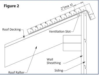
**STEP 4.** — It is very important that the Omni-Wall<sup>TM</sup> Vent be aligned correctly and evenly down the roof's peak. Place the first piece of the Omni-Wall<sup>TM</sup> Vent on the roof decking as intended to be installed. Mark the shingles at the location of the lower edge of the vent. Repeat this on the other end. Snap a chalk line down the roof and use the chalk line to help keep the OW-4 Vent straight and parallel to the roof peak.
