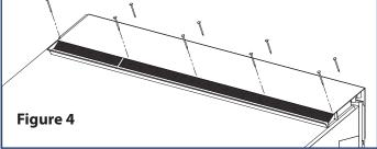
remaining vents ensuring the ends overlap properly. Take care to keep the vents as straight as possible while nailing. The last piece may have to be cut to the proper length. Be sure that the end plug is on the outside end of the last piece if the piece was cut. Seal the gap between the upper end of the accordion end plug and the flashing with a generous amount of sealant.
