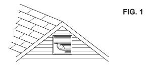
With the power vent installed, at least 780 square inches of inlet area must be provided. This is achieved by installing 12, 8" x 16" intake vents, measuring 65 square inches each. The inlet is best at the opposite end of the house to provide air flow the full length of the attic (Fig. 2). If your home needs more intake air, we suggest Lomanco Cornice or Soffit vents.
