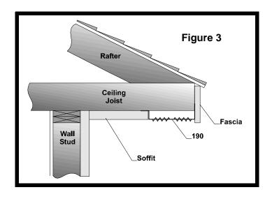
It must be noted that the 190 soffit vent will only ventilate your attic if it has a clear air passage, therefore it will be necessary to ensure that attic insulation as well as any other materials do not block your vents air passage.
