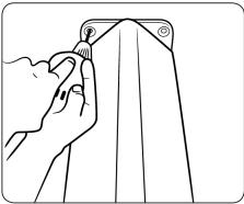
Repeat steps 2 and 3 for top of post using appropriate, installer provided fasteners, also must allow for countersink, and adjust the hole size from step 3 accordingly. Rotate post back to square with bottom plate.
