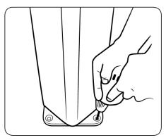
Pre-drill through bottom plate hole into bottom surface, secure (hardware not included, be sure to allow for countersink), and repeat with remaining 3 holes.
