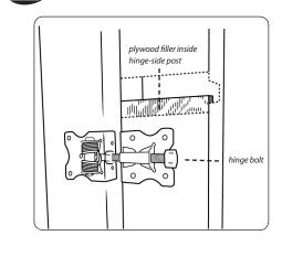
ezTIP: Before installing hinges, determine which way you want gate to swing. Hinges and latch striker will be mounted on the same side of gate posts.
