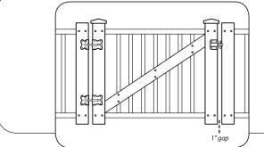
Hang gate so that there is a 1" opening on latch side of the gate. This can be accomplished by tightening or loosening the nuts on the T-Rod on the hinges. BOTH nuts on the T-Rod MUST be tightened or loosed together. Attach latch to the post to receive the latch striker.
