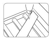
Insert 2 screws and screw caps through brace into center picket and pickets closest to posts. Be sure to not over tighten!
