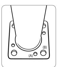
Note: Surfaces that the post is mounted on may vary, such as concrete, wood, composite decks or other surfaces. Always use appropriate installer provided hardware for your application.
