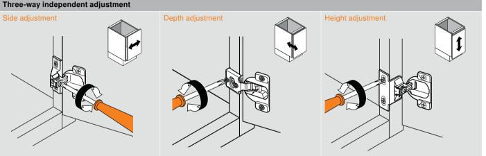
Side adjustment is possible on all COMPACT hinges except 38. series. COMPACT 38N, 38C and 39C have cam side adjustment.
