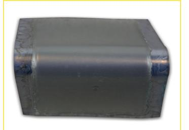
Through the Roof!® after 2000 hours of UV exposure. It's still clear, elastic, and adhering well. The result? A roof protected from leaks.
