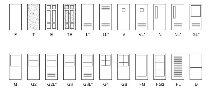
\* Add suffix I to indicate inserted louver Add suffix P to indicate pierced louver Add suffix A to indicate air condition grille
