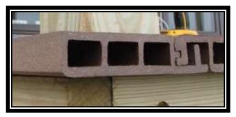
If the board is being placed against the house a minimum 1/8" gap should be allowed between the length of the board and the wall. A 1/8" gap should also be allowed at the point where the end of the board meets the house.
