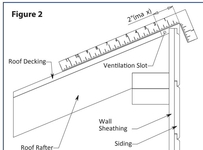
**STEP 4.** — It is very important that the Omni-Wall™ Vent be aligned correctly and evenly down the roof's peak. Place the first piece of the Omni-Wall™ Vent on the roof decking as intended to be installed. Mark the shingles at the location of the lower edge of the vent. Repeat this on the other end. Snap a chalk line down the roof and use the chalk line to help keep the OW-4 Vent straight and parallel to the roof peak.
