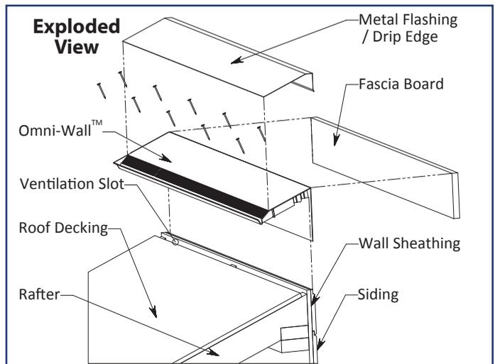
remaining vents ensuring the ends overlap properly. Take care to keep the vents as straight as possible while nailing. The last piece may have to be cut to the proper length. Be sure that the end plug is on the outside end of the last piece if the piece was cut. Seal the gap between the upper end of the accordion end plug and the flashing with a generous amount of sealant.
