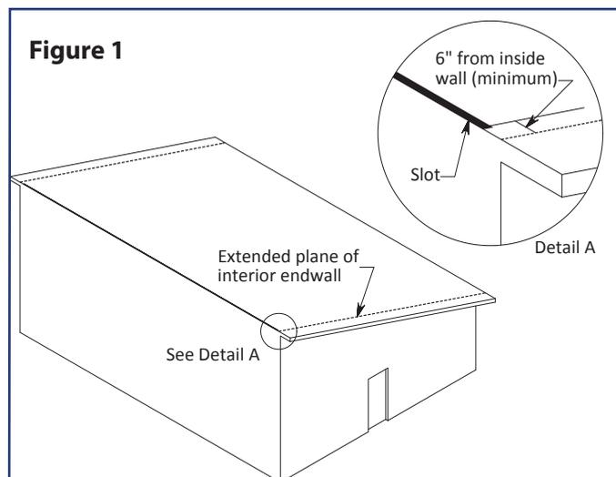
**NOTE: The decking should be cut parallel to the peak of the roof to ensure proper width of the ventilation slot.**
