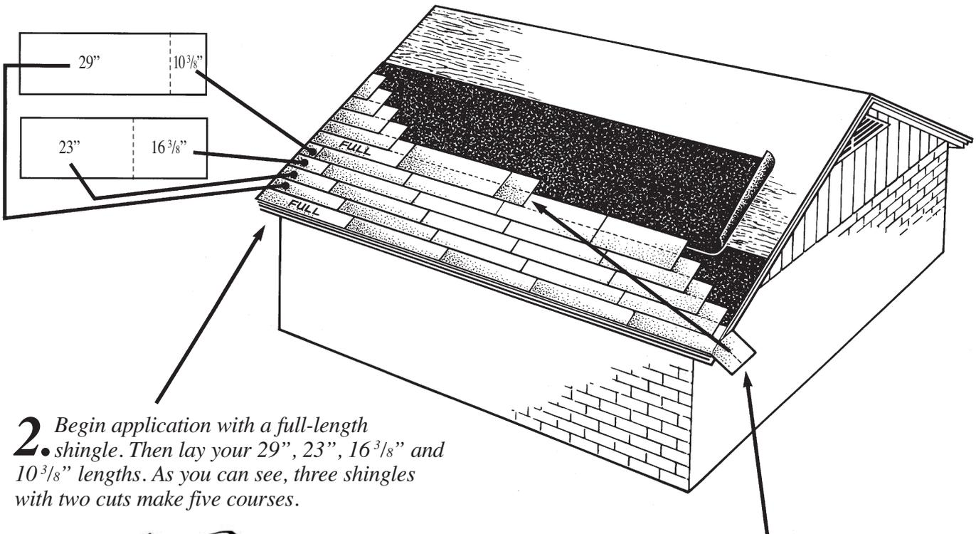
**2.** *Begin application with a full-length shingle. Then lay your 29", 23", 16<sup>3</sup>/<sub>8</sub>" and 10<sup>3</sup>/<sub>8</sub>" lengths. As you can see, three shingles with two cuts make five courses.*
